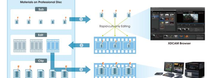
High-resolution data, Proxy Data, and the Clip List are separately recorded (to the Clip folder, Sub folder, and Edit folder, respectively). There are also a General folder and a User Data folder, both of which can be used to record any type of PC file.
