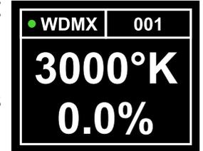
Wireless DMX dot is red when no signal is received, green when the MAXI Switch is connected to a Wireless DMX emitter.
