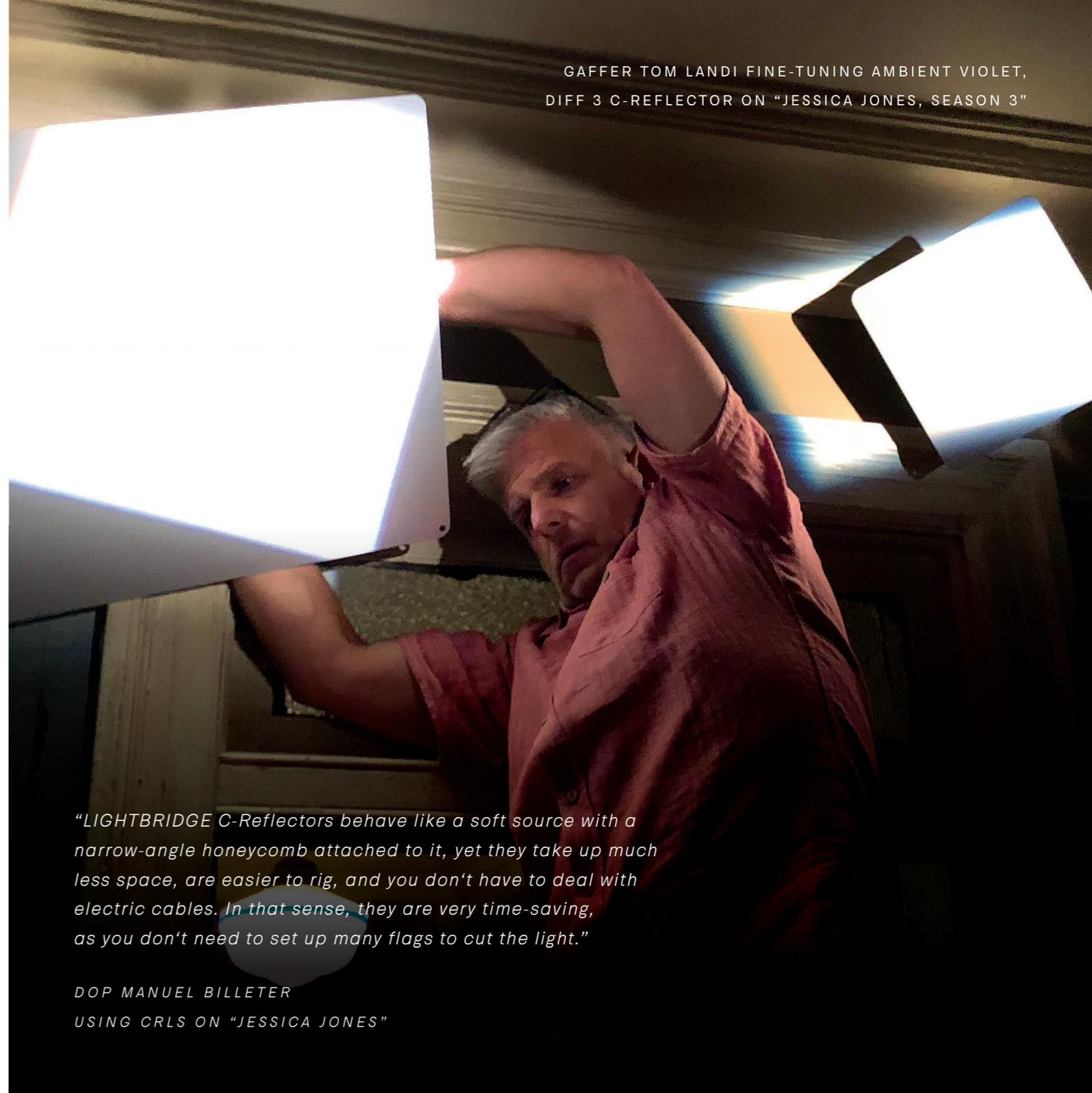
*"LIGHTBRIDGE C-Reflectors behave like a soft source with a narrow-angle honeycomb attached to it, yet they take up much less space, are easier to rig, and you don't have to deal with electric cables. In that sense, they are very time-saving, as you don't need to set up many flags to cut the light."*
