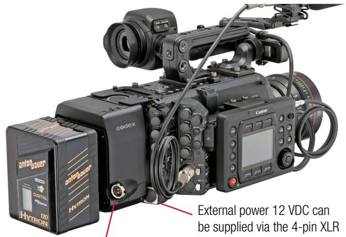
External power 12 VDC can be supplied via the 4-pin XLR connector on the camera.
