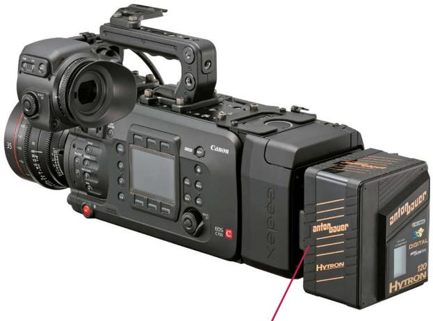
3. The rear of the Codex recorder has a battery plate to which an onboard Gold Mount Anton Bauer or V-Mount battery can attach (2 models).
