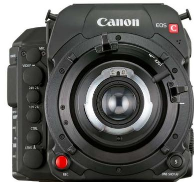
Canon C700 comes with the choice of two mounts. The Cinema Lock EF is a more rugged mount than the ones found on still cameras. This one has a locking ring and supports bigger, heavier lenses. FFD=44 mm. ID=54 mm.
