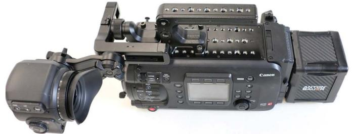
4. Top Handle attaches with 2 screws. OLED EVF-V70 comes with an adjustable support and cold shoe mount. (Note: the Anton Bauer Cine 150 battery shown here is V-Mount.)
