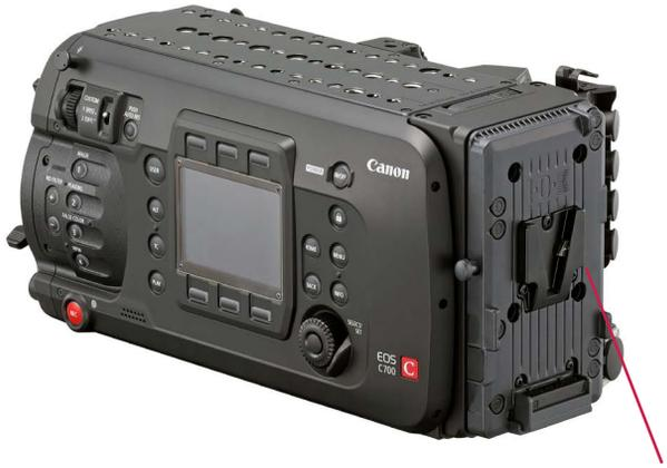
1. To attach the Codex CDX-36150, first remove the battery plate at the rear of the C700.
