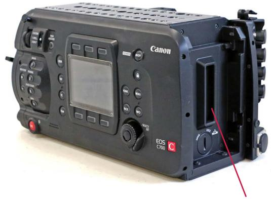
2. A multi-pin connector is revealed. The Codex Recorder connects here. CDX-36150 records 4K RAW uncompressed up to 120 fps.
