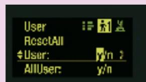
The drive unit can memorize 9 patterns of user-customised settings and also transmit the data between different drive units.
