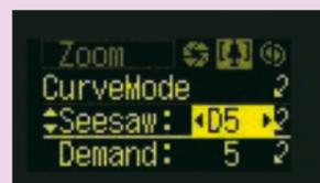
One of several operational curves can be chosen, which will allow different zoom movement characteristics when operating the seesaw switch. This is accomplished as a linear adjustment as opposed to an adjustment done in steps.
