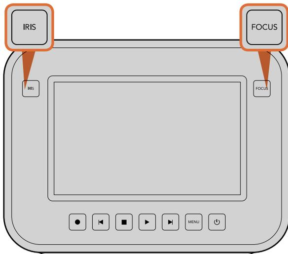
On Cinema Camera and Production Camera 4K, press the IRIS button, then use the transport controls to adjust aperture control. Press the FOCUS button for focus peaking.
