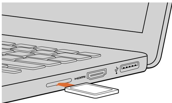
Insert your SD card into any computer with an SD card slot to access your clips immediately.
