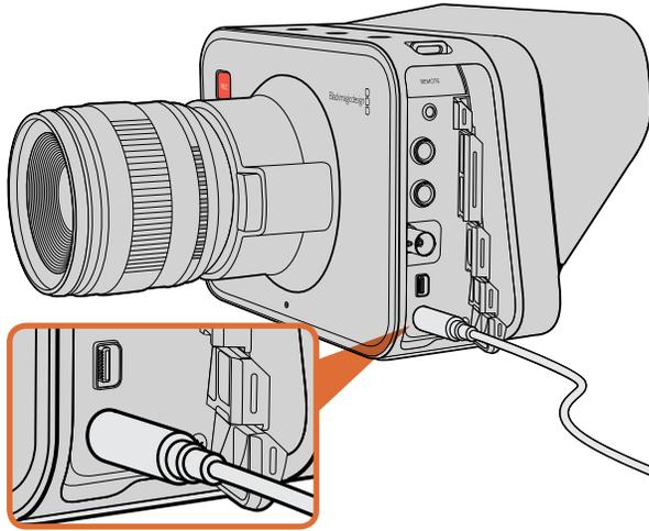
Use the supplied DC adapter to charge the internal battery and power the camera.
