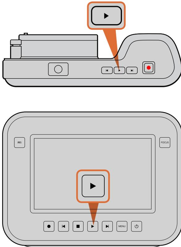
To immediately view your recorded clip on a Blackmagic Camera simply press the Play button on the transport controls.
