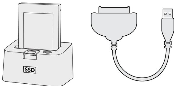
Edit directly from the SSD by removing it from your camera and mounting it on your computer using an eSATA Thunderbolt dock or USB 2.0 docking cable.
