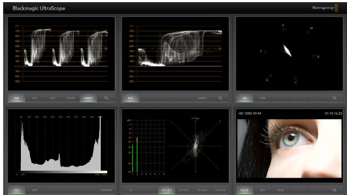
Blackmagic UltraScope software gives you accurate waveform monitoring via Thunderbolt.
