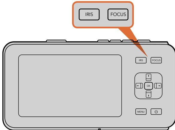
On Pocket Cinema Camera, press the IRIS button, then use the up and down directional buttons to adjust aperture control. Press the FOCUS button for focus peaking.
