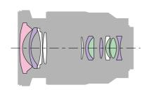
Advanced aspherical lens (AA lens)
