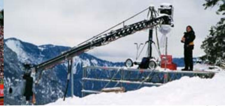
now offers eight possible length variations, and even at the longest reach, the Super Javelin MK II will comfortably support 40 kilograms / 88 lbs. The Stabilizing Bars on the front sections are situated on the side of the crane arm structure. This significantly reduces the overall surface
