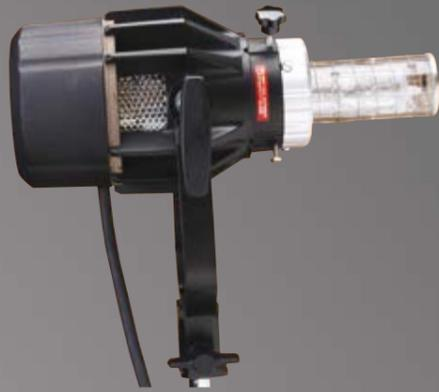
An 800W UV-Block lamp was designed at K5600 Lighting's request. The UV coating prevents the dispersion of harmful UV allowing the use of perforated safety globes. The Joker Bug 800 wattage was chosen to complete a range with a logical one stop increase between each model. In a lightbank the 800 W Bug-Lite gives more output and a better spread than a regular PAR 1200 W.
