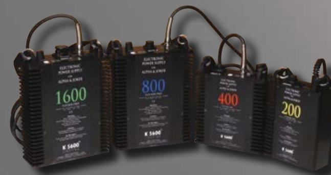
Resulting from a long relationship with Powergems, we designed a series of dedicated ballasts for our units up to 1600 W. Benefiting from the latest low frequency technology, the ballasts are smaller, run cooler, allow operation between 90 V to 265 V.
