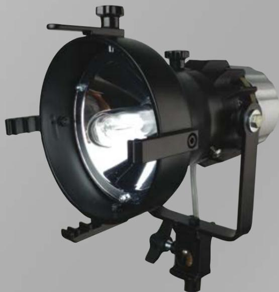
Why the Joker Bug 200 Evolution ? The difference between this one and the existing Joker Bug 200 is the fact that this program uses a different bulb. The LCL 200 W bulb made by SLI is slightly longer than the regular single-ended 200W MSR. Why change then? Because this bulb comes in two different color temperatures: 5600K and 3200K. They are both discharge lamps and feature a high lumen per watt ratio providing 4 times more light output than a tungsten bulb.
