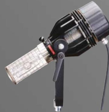
The 1600 Bug-Lite has no optics. Its bare-bulb output is optimal for use in lightbanks and lanterns, creating perfectly even distribution within such accessories whatever the size (from Small to Large) and shape (Rectangular, Octapuls, Strips...). The fact that the bulb is inside the diffusion tool eliminates hot spots and maximizes output. It can be used pointing straight down. There is no other lighting fixture on the market as versatile and user friendly than the Bug Lite 1600.
