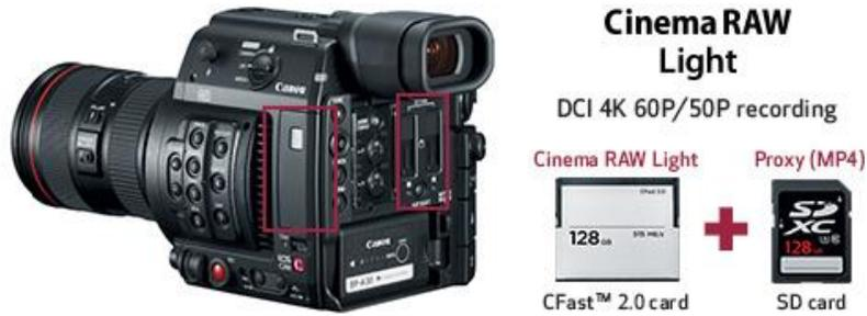
Cinema RAW Light files are about 1/3 to 1/5 the size of our standard RAW files. The smaller file size and reduced bit rate speeds up data transfer and allows internal recording to CFast™ cards.
