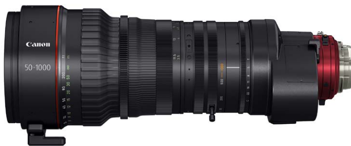
2014: 50-1000 mm T5.0-8.9 Zoom Length: 15.95 in. / 405.2 mm EF and PL Mount Weight: 14.55 lb / 6.6 kg Front Diameter: Ø 136 mm Image circle: 31.4 mm
