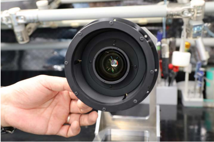
Assembling the optical elements inside the lens barrel.
