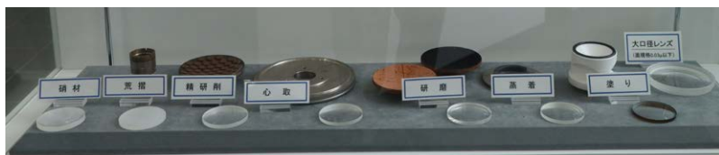
Display cases Utsunomiya Lens Factory lobby showing the stages of lens production.
