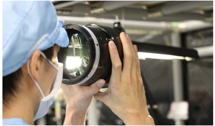
Assembling the optical elements inside the lens barrel.
