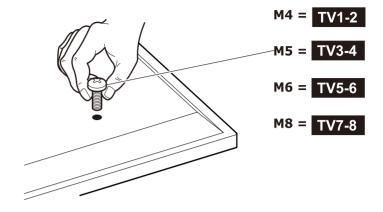
You are provided with 4 diameters of TV fixing screws, **M4**, **M5**, **M6** and **M8**. Determine the screw diameter that fits.
