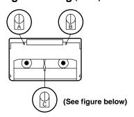
Use a screwdriver to push down the accidental erasure prevention pins, turn them 90° clockwise, and then lift the screwdriver to set the pins at their "down" positions.
