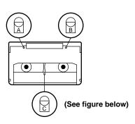
Use a screwdriver to push down the accidental erasure prevention pins, turn them 90° counterclockwise, and then lift the screwdriver to set the pins at their "up" positions.
