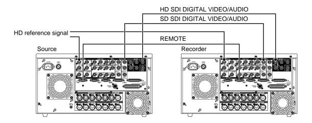
•When matching the CF (color frame) of SD output and time code output phase, also make SD reference matching. Then select SD REF as the OUT REF setting on the HOME SET UP menu.
