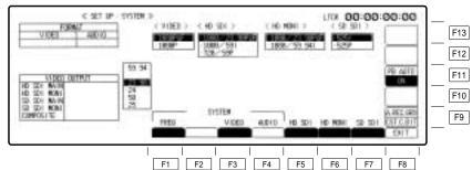
The frequency setting is possible when the F1 key is pressed. Select the frequency by cursor keys  $[\blacktriangle, \blacktriangledown]$  and press the ENT key, then the frequency is secured. In 59 Hz mode, the selection window will be further displayed (1080i/525i/720p). Select the format by the cursor key, and press the ENT key to secure the format. Then, select its 4-channel or 8-channel audio version, and enter the format by pressing the ENT key.
