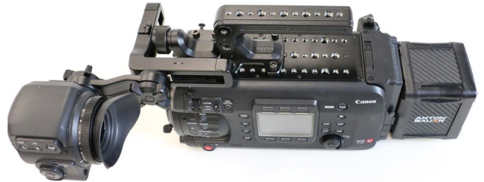
4. Top Handle attaches with 2 screws. OLED EVF-V70 comes with an adjustable support and cold shoe mount. (Note: the Anton Bauer Cine 150 battery shown here is V-Mount.)
