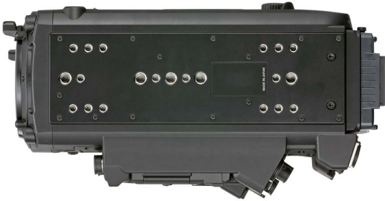
3. Bottom mounting plate. Lots of 3/8-16 and 1/4-20 threads.
