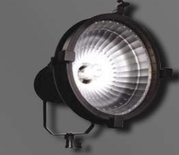
The ballast of the 1600 is PFC and draws 7,4 Amp @230 V. It is dimmable, and has selectable frequency options for extreme High Speed shooting (300 Hz and 1000 Hz).
