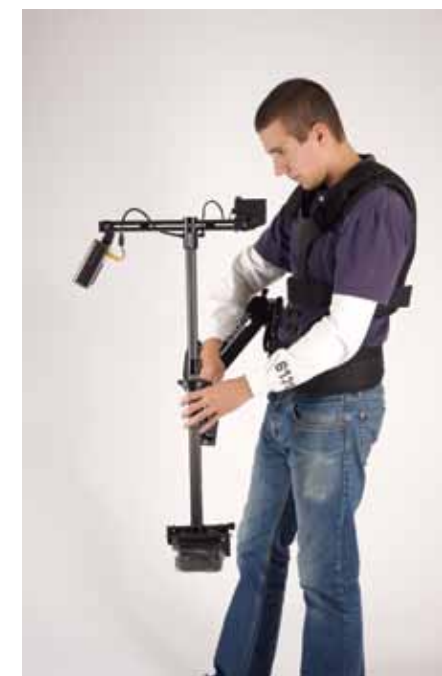
With the camera right side up in low mode, you must rotate the Pilot's monitor above the spar as shown in the photo.
