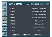
This product provides a REMOTE CONTROL mode. The user may connect RJ-45 jack to the REMOTE terminal on the rear of the unit and designate a function for each pin.
