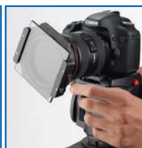
Filter Holder with Linear Polarizer is rotated to achieve desired ND setting
