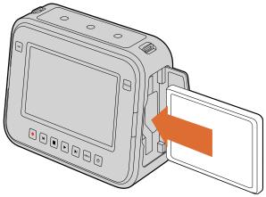
Inserting a SSD into the Cinema Camera and the Production Camera  $4\mathrm{K}$
