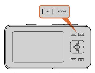
On Pocket Cinema Camera, press the IRIS button, then use the up and down directional buttons to adjust aperture control. Press the FOCUS button for focus peaking.
