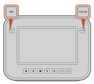
On Cinema Camera and Production Camera 4K, press the IRIS button, then use the transport controls to adjust aperture control. Press the FOCUS button for focus peaking.
