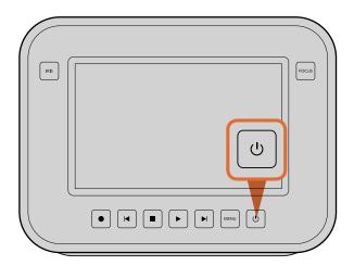
Press and hold the power button to turn the camera on or off.
