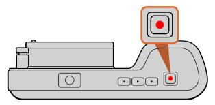
Press the REC button on the top of Pocket Cinema Camera
