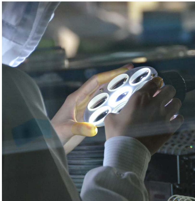
Large vacuum deposit machines coat the lenses with an antireflective (AR) coating that improves contrast, reduces light loss, glare and flare.
