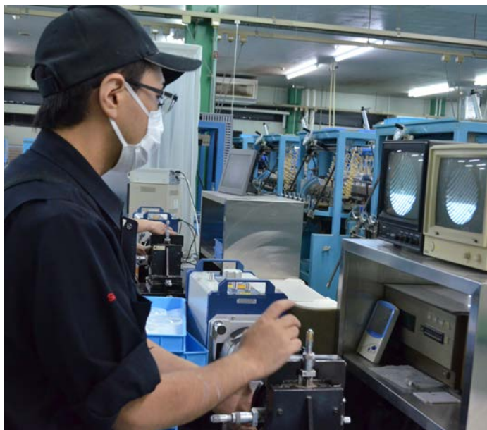
Checking spherical elements on an interferometer
