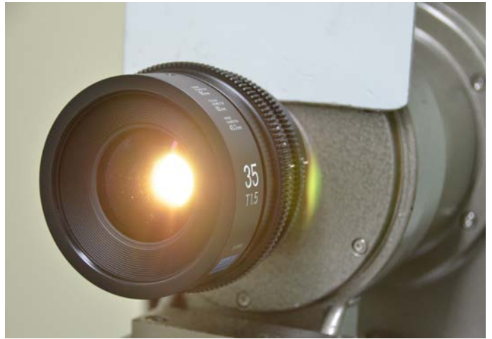
A new 35mm T1.5 Sigma Cine lens is tested on the projector
