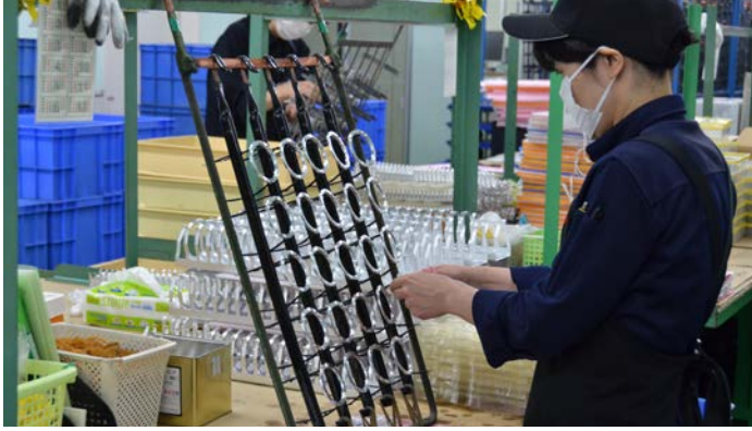
Aluminum parts are prepared on trays prior to anodizing
