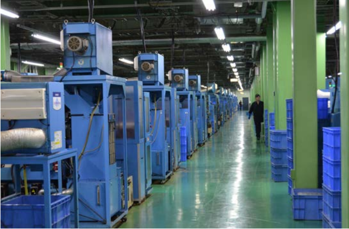
A forest of CNC machines craft mechanical parts like lens barrels. Engineers load the designers' plans into computers that guide the machines.
