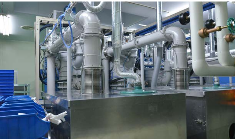
Large vacuum deposit machines coat the lenses with an antireflective (AR) coating that improves contrast, reduces light loss, glare and flare.
