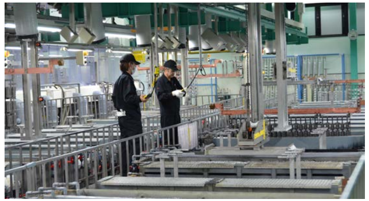
Anodizing is done on a vast scale in house in many colors and shades
