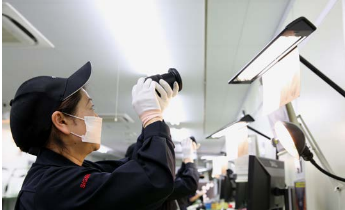
Each finished lens is hand inspected and tested on its intended camera
