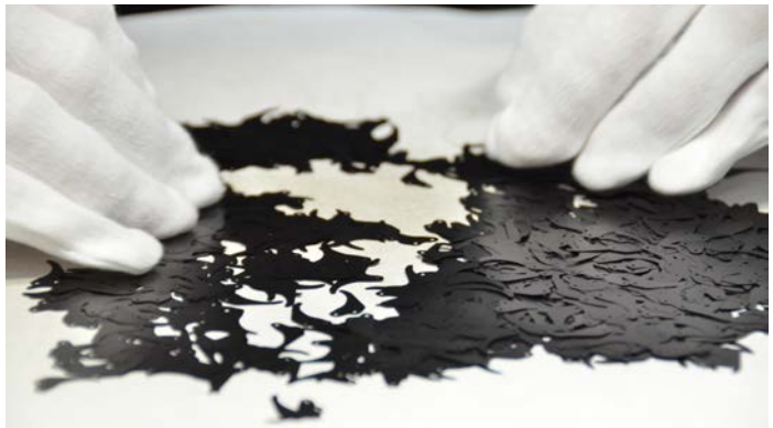
The iris leaves are anodized, sorted and assembled by hand
