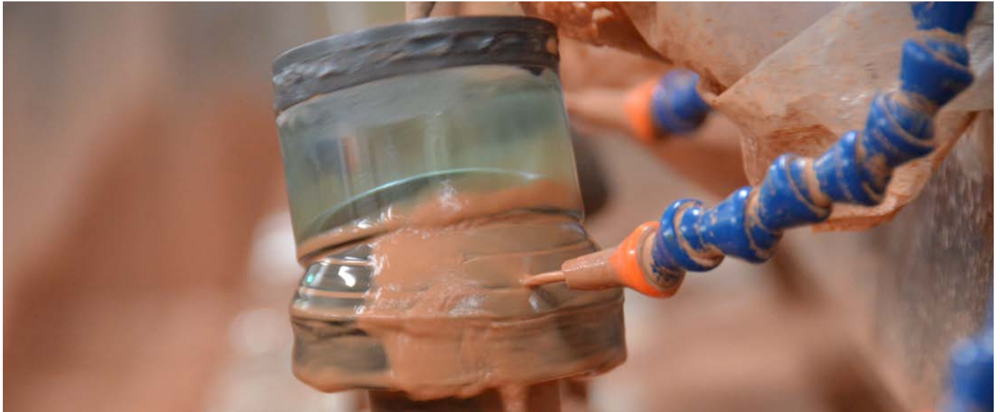
Traditional lens polishing of spherical elements in a vast “analog” machine room at the Sigma Aizu factory
