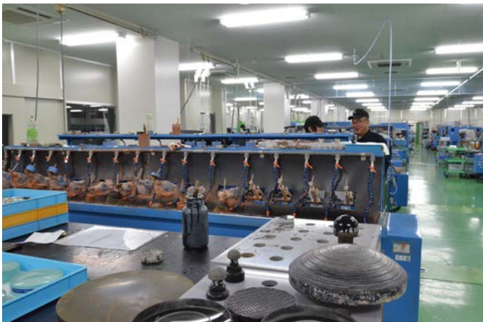
Traditional lens polishing of spherical elements in a vast “analog” machine room at the Sigma Aizu factory
