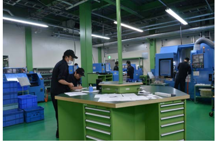
A forest of CNC machines craft mechanical parts like lens barrels. Engineers load the designers' plans into computers that guide the machines.
