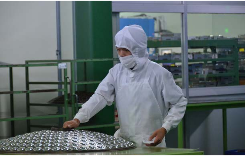
Preparing the optical elements in large trays prior to coating
