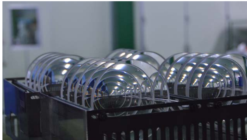
Large vacuum deposit machines coat the lenses with an antireflective (AR) coating that improves contrast, reduces light loss, glare and flare.
