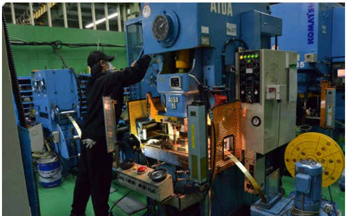
Even with CNC machines, some parts are still made "the old-fashioned" way. At right: long bands of metal are cut into shape to make lens irises.
