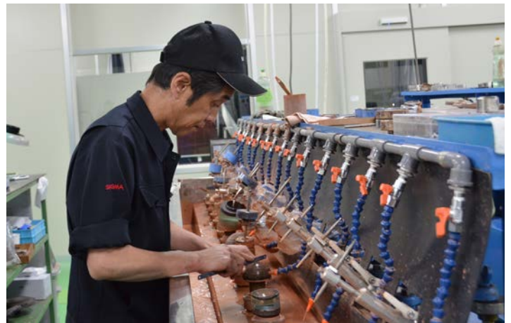
Traditional lens polishing of spherical elements in a vast “analog” machine room at the Sigma Aizu factory
