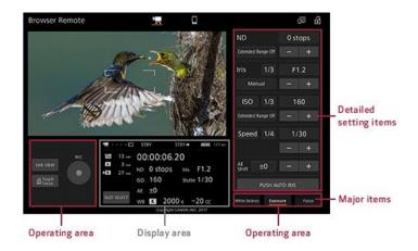
A wide range of auto focus functions can also be controlled using the Browser Remote, including the ability to move the focus area with just a touch when using a compatible tablet or smartphone.
