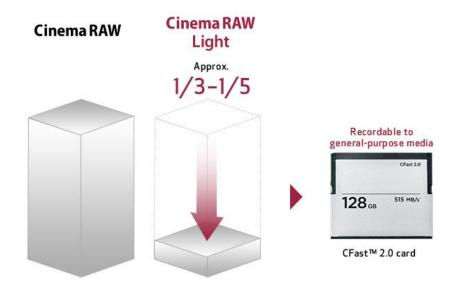
The reduced file size also helps users extend storage capacity and transfer files on a network more easily. The high bit depth of Cinema RAW Light (10bit/12bit\*<sup>2</sup>) maximizes retention of color and dynamic range information, which is especially critical in HDR production.
