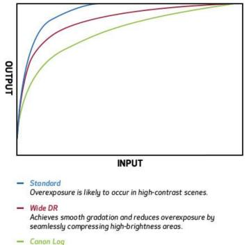
Enables color corrections with high flexibility because a sufficient margin is provided for high-brightness areas.
