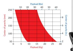
SPECIFICATIONS Max Payload capacity **22 Kg** 49 lbs 8.6 lbs 3,9 Kg 100mm / 150mm / Flat Bowl diameter ± **90**° Tilt range 360° Pan range Counterbalance Continuous Fluid Drag Continuous Euro-style quick release Temperature range -40°/+60° C -40°/+140° F
