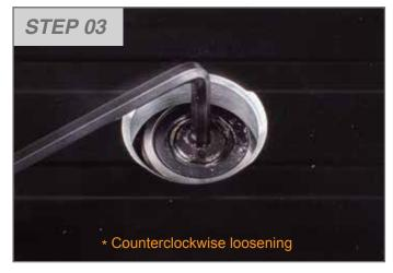
Use the hex wrench to unlock bearings. (Using hex wrench 2.5mm)
