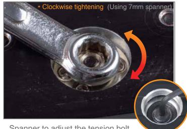
Spanner to adjust the tension bolt and bearing lock.
