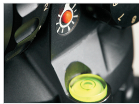
Illuminated levelling bubble.
